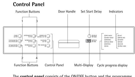
The **control panel** consists of the ON/OFF button and the programme buttons with LED displays.
